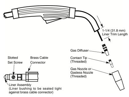
FIGURE D.2b Liner trim length for gun with <u>red trigger</u> (Magnum™ 100L)
