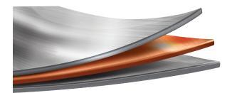
copper layer reduces the residual cooling tensile caused by the different expansion rates between the base metal (usually steel) and the segments (usually tungsten carbide).
