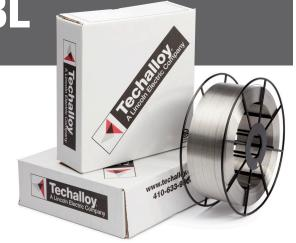
**Techalloy**® **308/308L** electrodes give a weld deposit, with reduced carbon levels (0.04% max) that offers increased resistance to inter-granular corrosion. Type 308L is ideal for welding Type 304L stainless steels.
