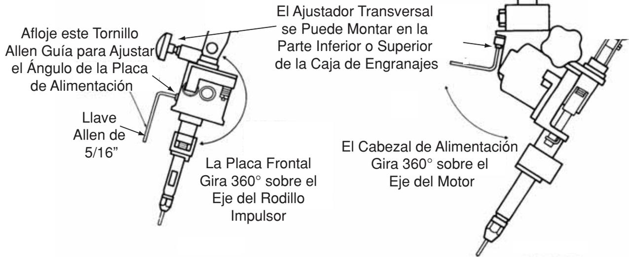
FIGURA B.2 – AJUSTE HORIZONTAL
