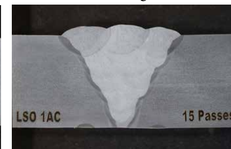
O sarma AC LSO (grosime 40mm)
