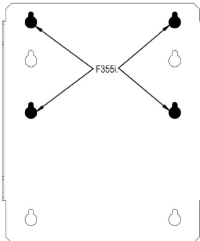
4. Pull the bracket toward the right of the F355i to engage the keyhole slots with the screws.
