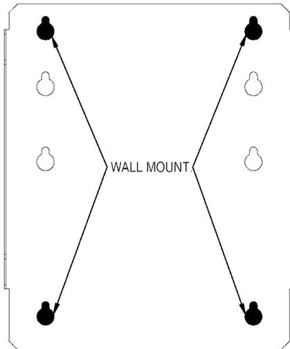
3. Start the fasteners into the drilled and tapped mounting holes leaving enough space between the heads of the screws and the mounting surface to clear the Mounting Bracket sheet metal thickness.
