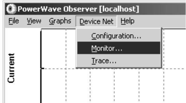
From the file menu select Device Net and then select Monitor. The DeviceNet Monitor will display the status of the connection and its data. If everything is operating correctly, the "Polled IO Cnx State" will display "Established" and the IO Scans/Sec will have a non-zero value. If there appears that there is no connection to the Power Wave refer to the trouble shooting section of this quick start guide.
