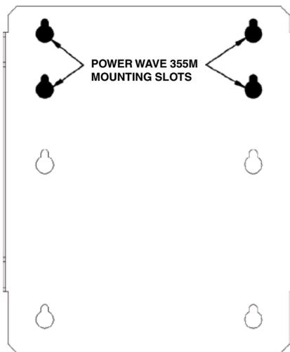
4. Pull the bracket toward the back of the Power Wave 355M to engage the keyhole slots with the screws.
