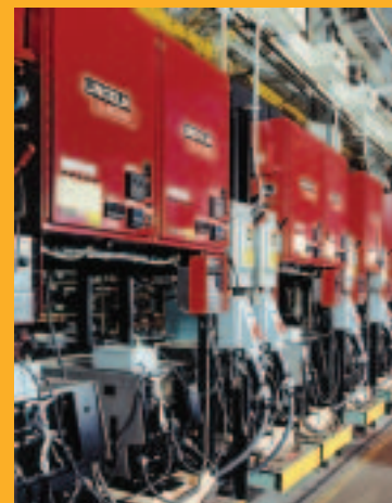
The burn-in cycle is conducted to ensure machine performance matches Lincoln Electric requirements.
