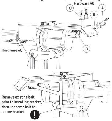
**Step 3**Install the Wire Feeder.
