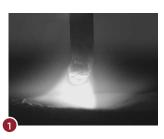
**PULSE RAMP/PEAK** A rapid current increase creates a molten droplet.
