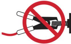
The work sense lead should be separated away from welding cables to minimize interference.
