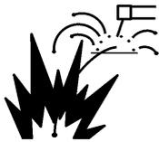
**CUTTING SPARKS can cause fire or explosion.**
