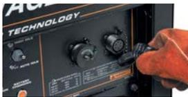
Output automatically switches to remote mode when remote device is connected. For the CC-stick, downhill pipe and Touch Start TIG modes, the machine output dial becomes a maximum current limit for more fine tuning with the remote control dial or Amptrol™.
