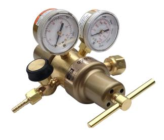
This unique two stage regulator is specifically designed for  $CO^2$  service to provide gas to incubators. This two stage design reduces the occurrence of  $CO^2$  freezing due to the Jules Thompson effect. This regulator has a cartridge seat assembly to provide better flow characteristics and long life.
