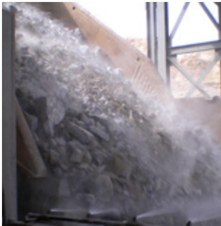
Exposure to extreme wear from sliding abrasion
