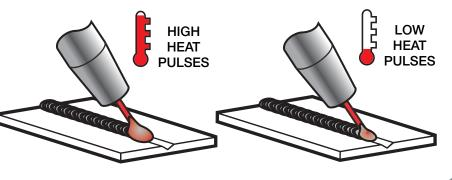
Pulse on Pulse™ (GMAW-PP) is a Lincoln patented process specifically designed for use in welding relatively thin (less than 1/4" thick) aluminum. It produces weld beads with very consistent uniform ripple.
