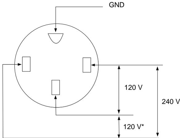
\*Current Sensing for Automatic Idle.
