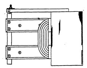
5. If shunt binds or sticks at all when moved back and forth along the guide then the guide is bent.
