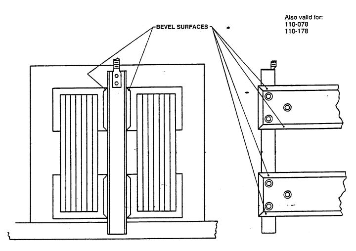
**END VIEW OF TRANSFORMER AND SHUNT**
