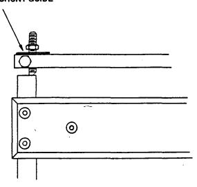
When tapping guide either up or down both sides must be tapped equally so that washer does not become cocked.
