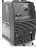
for this information. Then connect the output cables to the output terminals of the machine for the selected polarity. For example, if DC(+) welding will be used then connect the electrode cable to the (+) terminal of the machine and the work clamp to the (-) terminal. Insert the connector with the key lining up with the keyway and rotate approximately ½ turn clockwise. Do not over tighten.
