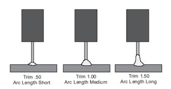
Most pulse welding programs are synergic. As the wire feed speed is adjusted, the Air Vantage® 600X PLUS will automatically recalculate the waveform parameters to maintain similar arc properties.
