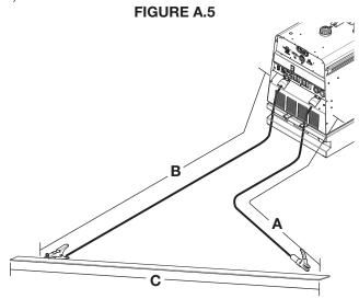
To minimize inductance always use the appropriate size cables, and whenever possible, run the electrode and work cables in close proximity to one another to minimize the loop area. Since the most significant factor in cable inductance is the welding loop length, avoid excessive lengths and do not coil excess cable. For long work piece lengths, a sliding ground should be considered to keep the total welding loop length as short as possible.
