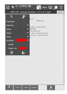
From the FANUC Plugin List ensure that Cooper\_App is highlighted. Scroll down on the page until the Uninstall button is shown. Click on "Uninstall" and then OK on the pop-up to confirm the uninstallation of the Cooper App. Note, the teach pendant will need to be enabled. Cycle power on the controller one the app has successfully been uninstalled by manually switching the controller off then turning it back on.
