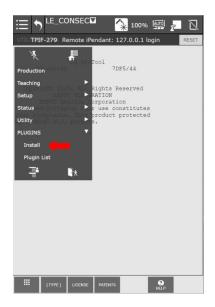
Verify that the version of the software to be installed is correct by referencing the Description -> Version. Once confirmed press Install -> OK buttons and wait for the install to complete. Note, the teach pendant will need to be enabled. The installation process will take a few minutes (5 - 10). The message "Plugin software successfully installed!" will be shown if successful. Cycle power on the controller by manually switching the controller off then turning it back on.
