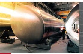
Versatile range of roller beds for the handling of circular pieces such as pipes, tubes, vessels or containers during welding operations, and to ensure continuous production and reliable performance.
