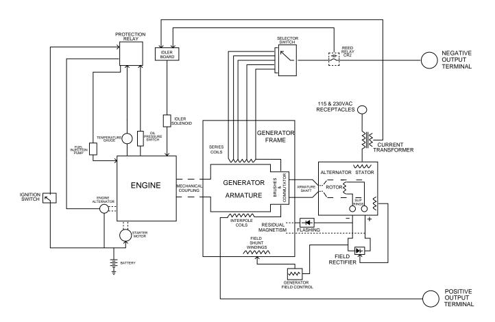
FIGURE E.1 - SA-250 BLOCK LOGIC DIAGRAM
