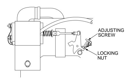
FIGURE F.9 - LOW IDLE ADJUSTMENT
