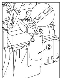
CHANGE THE OIL FILTER: Change the oil filter the first time between 25 and 50 hours of operation. Then, under normal operating conditions, change the oil filter after every 200 to 250 hours of operation. If the engine is operated under heavy load or in high ambient temperatures, change the oil filter more frequently. See Table D.1 for recommended maintenance intervals. Order Perkins oil filter #2654408 from your local Perkins service center.
