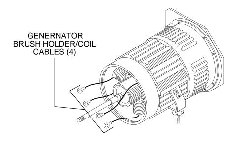
17. With the 1/2" wrench, disconnect and clear the four heavy cables from the generator brush holders to the coils in the generator frame. It is not necessary to remove the brush holder jumper cables. See Figure F.17. Label leads and positions for re-assembly.
