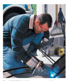
The SPEEDTEC® 200C is easy to set up. Select welding parameter by either manually setting Amp and volts, synergic or by selecting materials, wire diameter, shielding gas and material thickness.
