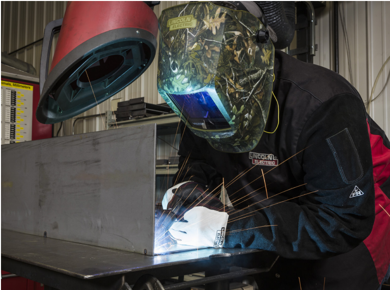
MIG welding a grill shelving unit.
