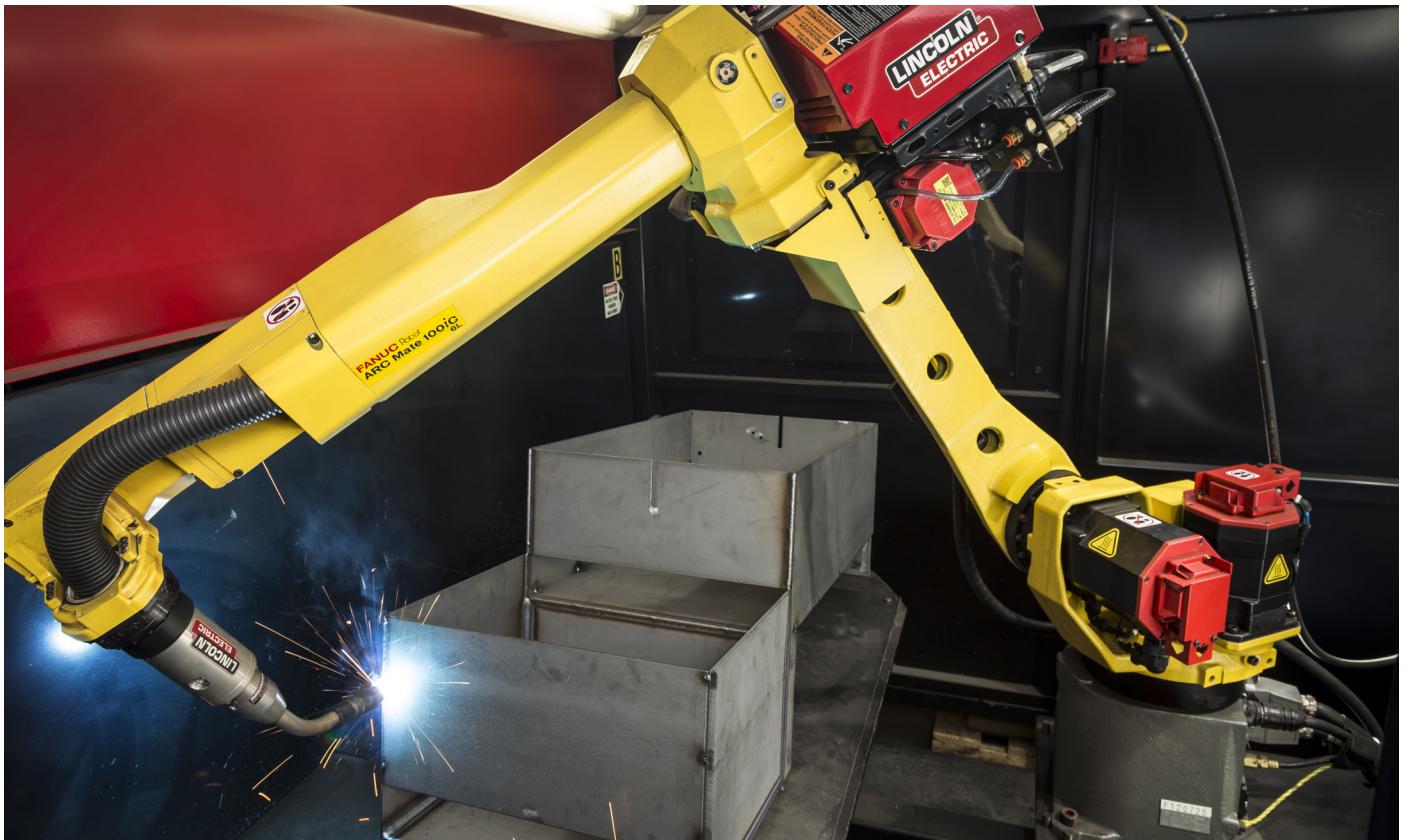
Robotic welding the grill hull for the 1000 Series Braten® grill using the System 40.
