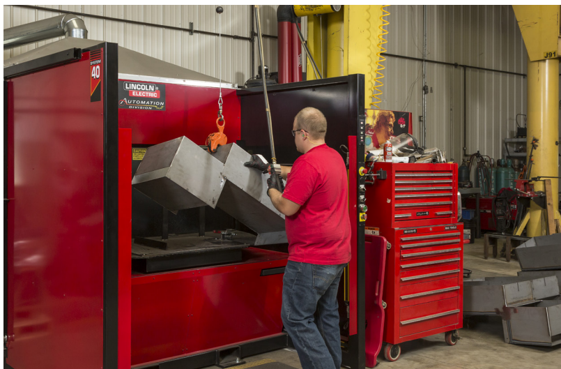
An Engelbrecht Grills & Cookers’ employee places a grill hull in a welding fixture.
