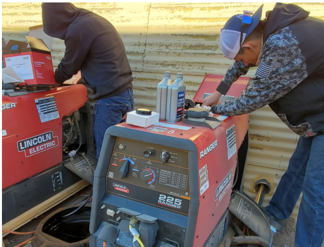
Welding students completing preventative maintenance on the welding machines they are using in class.
