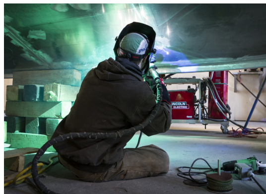
MetalCraft Marine personnel seam welding the hull of a work boat.
