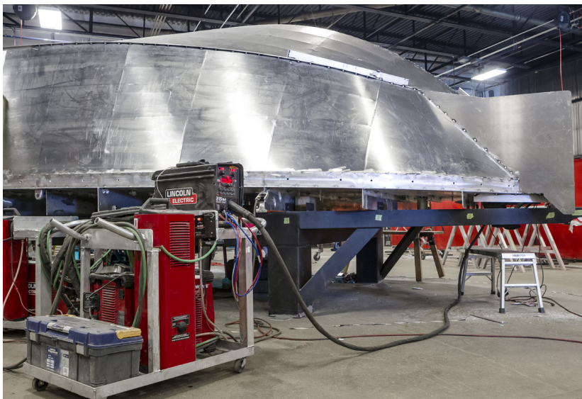
Constructing the hull of an aluminum high-speed patrol boat.
