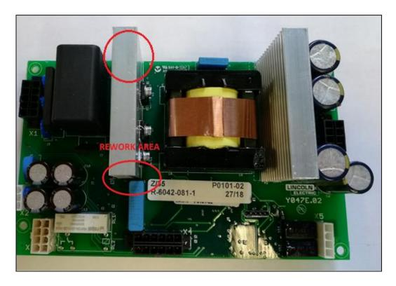
3. Uplift H1 heatsink slightly with a flat screwdriver – heatsink will tilt to right side (to transformer T1).
