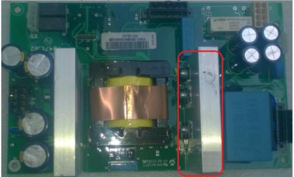
Missing an insulation paper under H1 heatsink:
