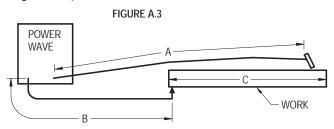
For long work piece lengths, a sliding ground should be considered to keep the total welding loop length less than 50 ft.(15.24m). (See Figure A.4.)
