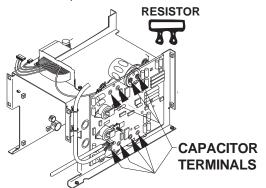
Use a DC voltmeter to check that voltage is not present across the terminals on all four capacitors.
