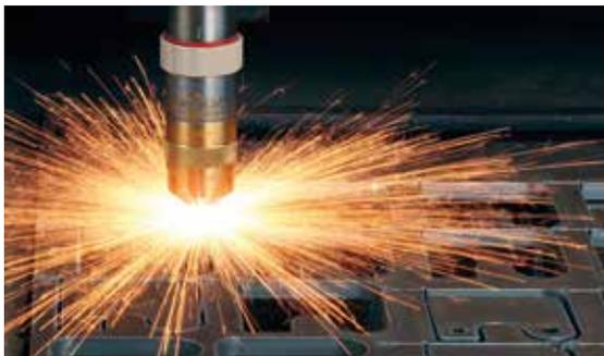
**During manual or automatic cutting** using gas or plasma, fumes are generated above the cut material and **therefore carried away from above the work surface.**
