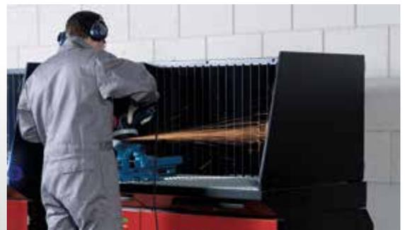
For optimum efficiency, it is necessary to adapt the speed of capture to the point of emission of fumes depending on the process used. Our team of fume control specialists will work on a solution that best meets your requirements.
