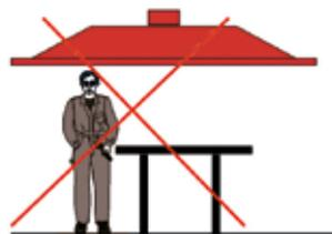
In that case, the operator's face would be located between the point of emission of fumes and the hood.
