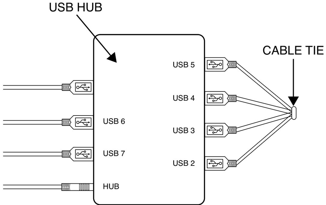
Figure B.114 – Patriot SEU module serial connection location
