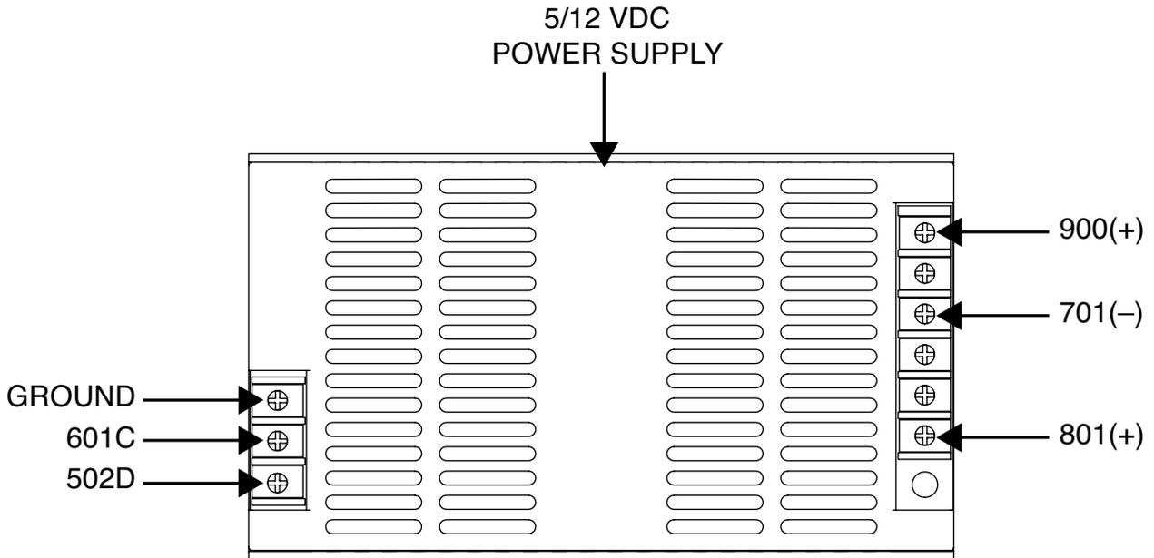
Figure B.55 – 5/12 VDC power supply mounting screw location
