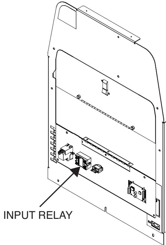
Figure B.70 – Input relay lead location
