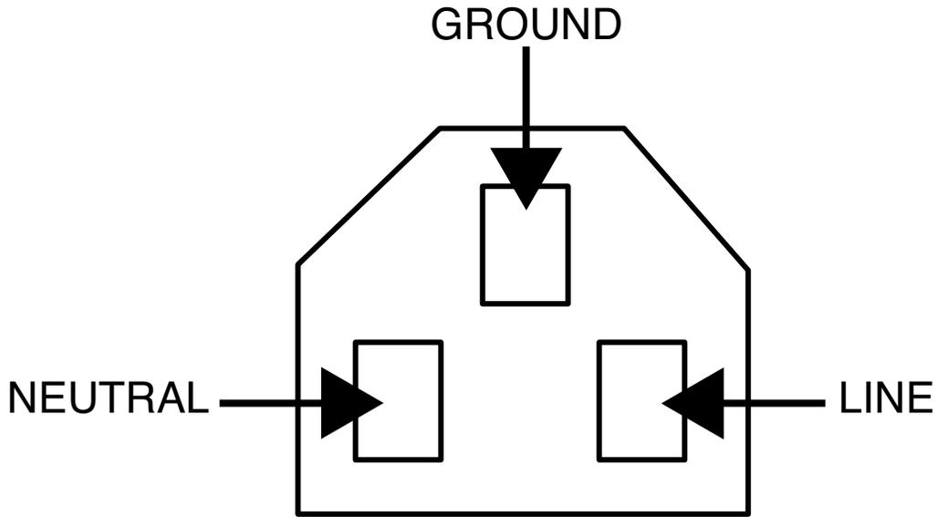
Figure B.21 – Input relay test points
