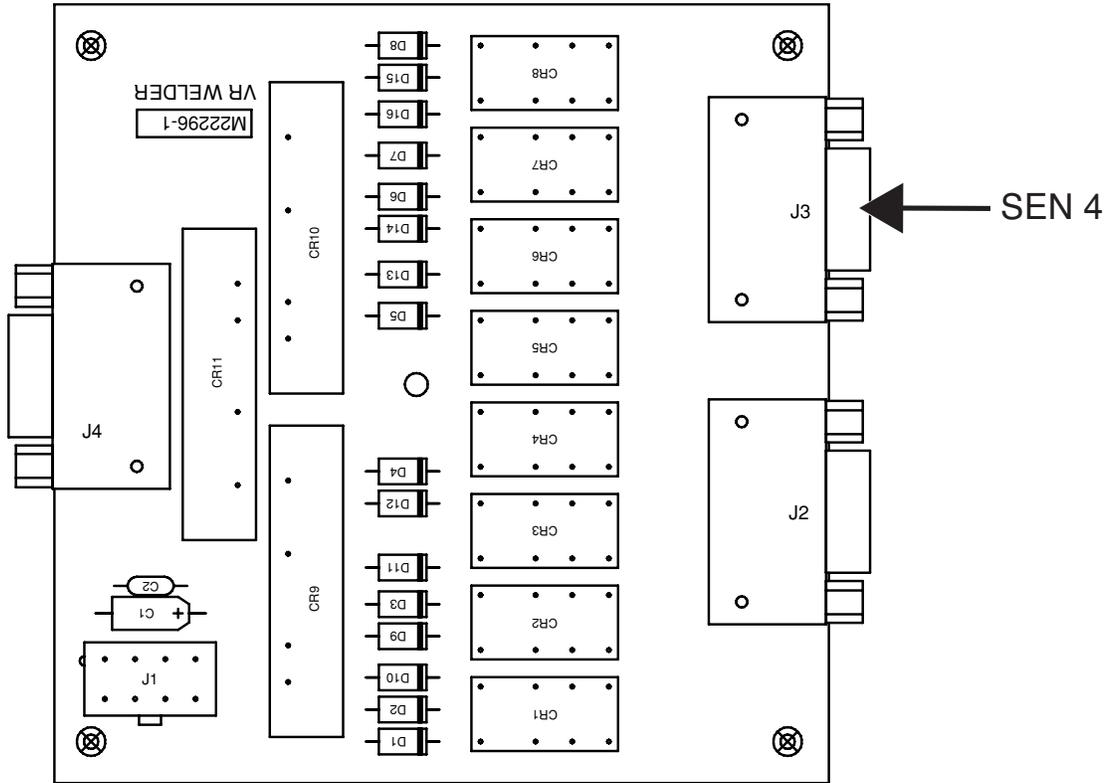
Figure B.110 – Input cable location
