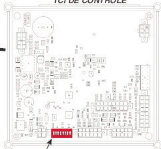
EMPLACEMENT DES INTERRUPTEURS DIP
