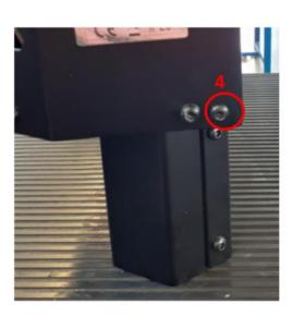
3. Slowly move back panel as it is shown in below photo and disconnect PE wire from the panel
