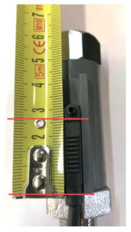
7. Tighten the hex screw of flow sensor and check that is not moving.
