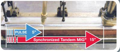
The maximum deposition rate in a traditional single wire GMAW (MIG) process is limited by the saturation current(I) for any specific wire diameter. To overcome this limitation, Tandem MIG combines two separate MIG welds into a single application. The outcome is a process capable of nearly double the deposition rate of single wire MIG.
